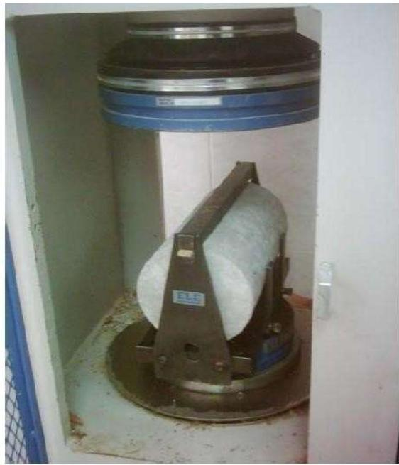
Figure: Cylinder in compression machine
