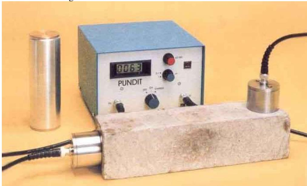
Figure 16: Ultrasonic Pulse Velocity Apparatus
