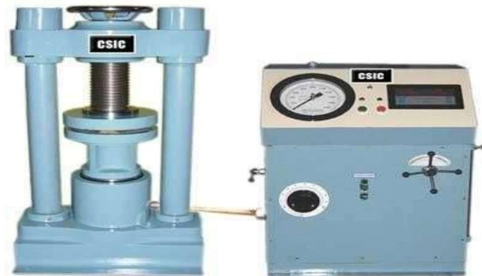
Figure: Cube Testing Machine
